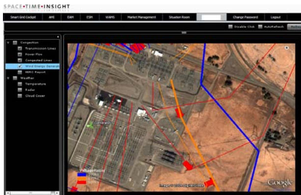
Screenshot of Space-Time Renewables Composite shows power flow and intermittency estimations to visualize potential grid congestion issues.
