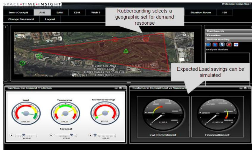
Users click the Space-Time Demand Response Composite screen to rubberband an area for demand response participant selection. Expected load savings can be simulated for the rubberbanded selection.
