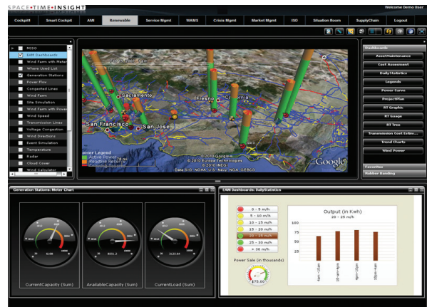
Screenshot of Space-Time Insight shows renewable energy generation in the context of grid congestion alerts, enabling improved renewables integration and grid balancing decision making.
