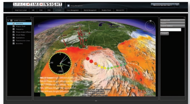
Screenshot of Space-Time Insight's Historical Replay feature showing phase angle differences of Phase Measurement Units (PMUs) in the path of a hurricane.
